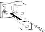
When removing the Serial Communication Module do so in reverse of the procedure shown above.
