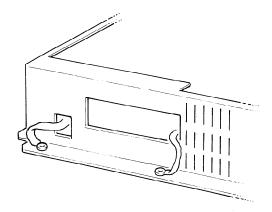
Install the FG mesh wire solderless terminal in the EMC Box's FG mesh wire ground area facing the normal direction.
