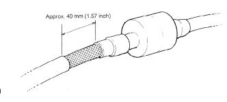
② Choose the respective cable clamps for the control panel in which the GOT is installed and the control panel in which the PC CPU is installed and ground the connection cable.
